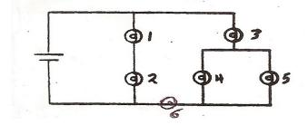
58. Given six resistors as shown to the left. The resistance of 1 is 1.0 ohm, of 2 is 2.0 ohm, of 3 is 3.0 ohm, etc. The equivalent resistance for the 6 resistors is \_\_\_\_\_ ohms.
