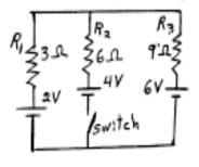
**43-44**, Given Resistors R1, R2, and R3 of 3 ohms 6 ohms, and 9 ohms, respectively, and three ideal emf's of 2 V, 4 V, and 6 V, respectively.
