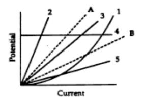
6. Given graphs of "Potential Difference as a Function of Current" for two resistors A and B. The dashed lines represent the data for A and B. If resistors A and B were placed in parallel, which of the 5 solid lines would represent the data for the parallel combination? \_\_\_\_\_. A) 1 B) 2 C) 3 D) 4 E) 5
