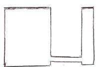
Given a Pascal's Principle device, a hydraulic lift. Two circular cylinders of equal height stand next to each other and are joined near their bottoms by a small tube. The tube is 0.02 m in diameter. The cylinders are 0.40 m tall. The cylinders and the tube are filled with water. They each have essentially friction free "massless" pistons at their tops. The diameter of the
