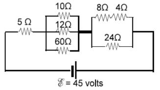
Given seven resistors arranged as shown to the left, 5, 10, 12, 60, 8, 4, and 24 ohms. They are connected to an emf listed as 45 volts.
