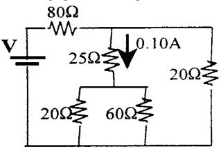
Given a circuit of five resistors connected to a potential difference, V . The current through the 25 ohm resistor is 0.1 ampere, as shown.
